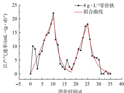
图 3  $4 \text{ g} \cdot \text{L}^{-1}$  零价铁投加量下的产气速率变化Fig. 3 Change of gas production rate with the addition of  $4 \text{ g} \cdot \text{L}^{-1}$  zero valent iron
